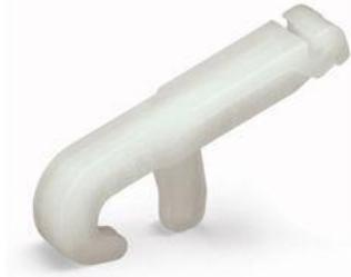
The hook gets attached into the upper opening, which is situated above the cable locks. Then, by applying pressure on the hook downwards, the locks will open enough for the stripped cable to be put in.
